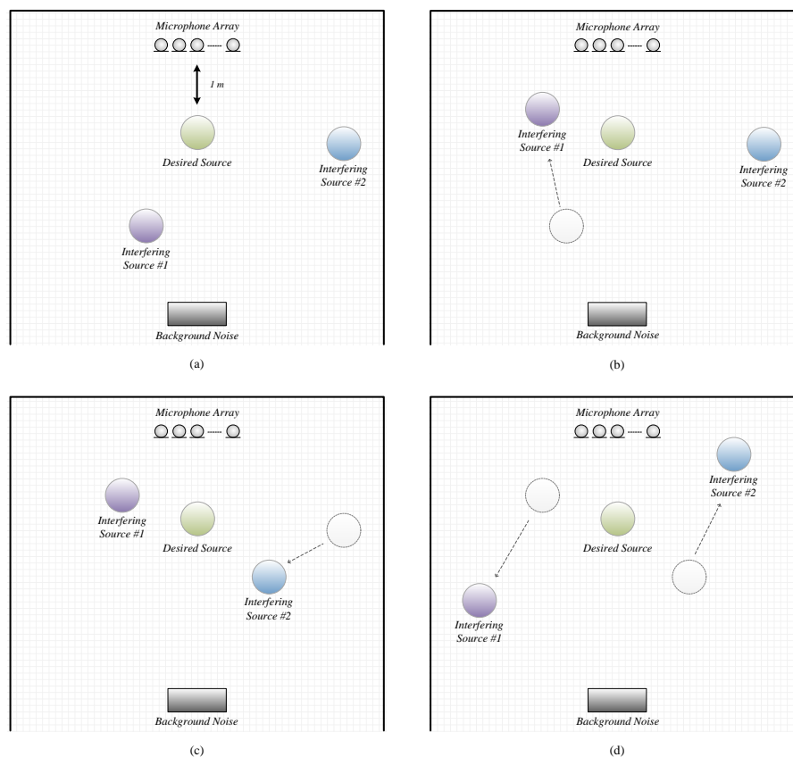
Fig. 5: Second configuration. (a) 0-5 seconds: initial positions (same as first configuration); (b) 5-10 seconds: position change of the first interfering source; (c) 10-15 seconds: position change of the second interfering source; (d) 15-20 seconds: simultaneous position change of both the interfering sources.
