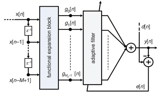
Fig. 1 Functional link adaptive filter
