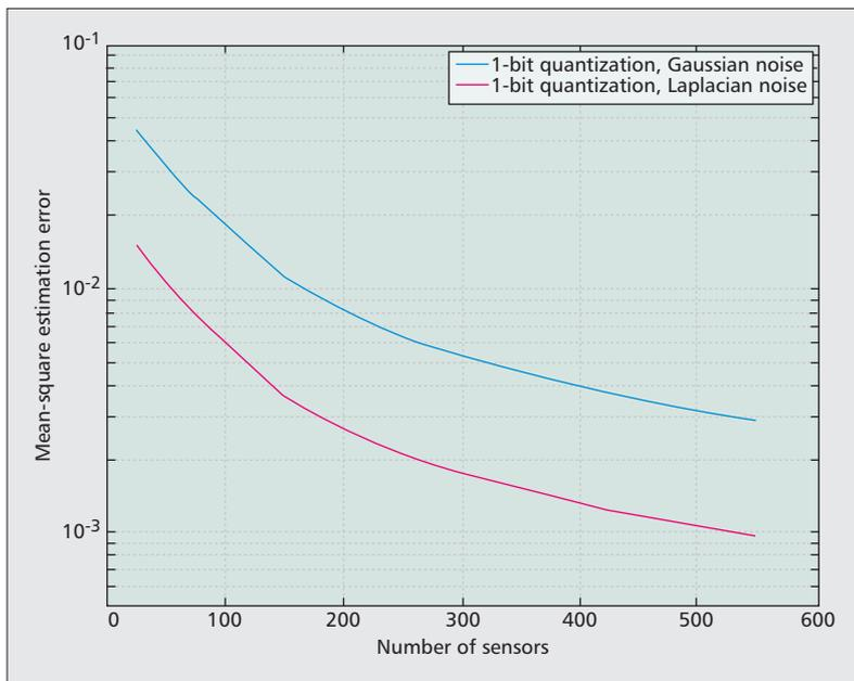
**Figure 3.** Example of optimal fusion mean square error parameter estimation performance for a dense MWSN assuming 1-bit quantization in the presence of Gaussian or Laplacian noise [6].
