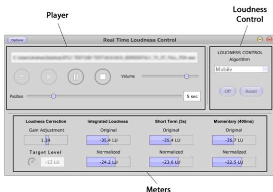
Figure 2 Controller GUI
